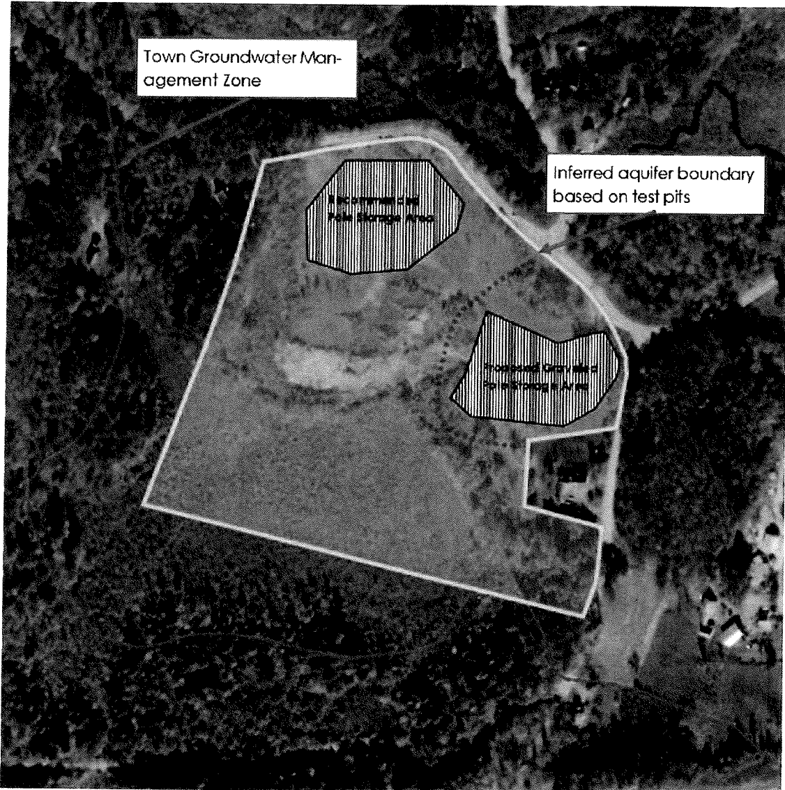
Figure 3: Approximation of proposed and recommended utility pole storage areas. Yellow shading indicates the approximate property area. The mapping source is the New Hampshire Department of Environmental Services (NHDES) On-line Data Mapper.
